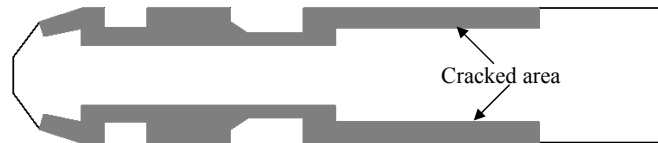
Figure 6. Assumed cracked area beneath the pier
