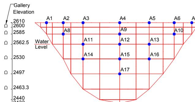
**Figure 2. Accelerometers used to measure dam response**
