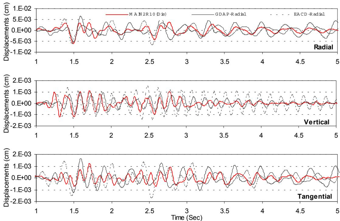
**Figure 9. Comparison of measured and predicted crest displacements**
