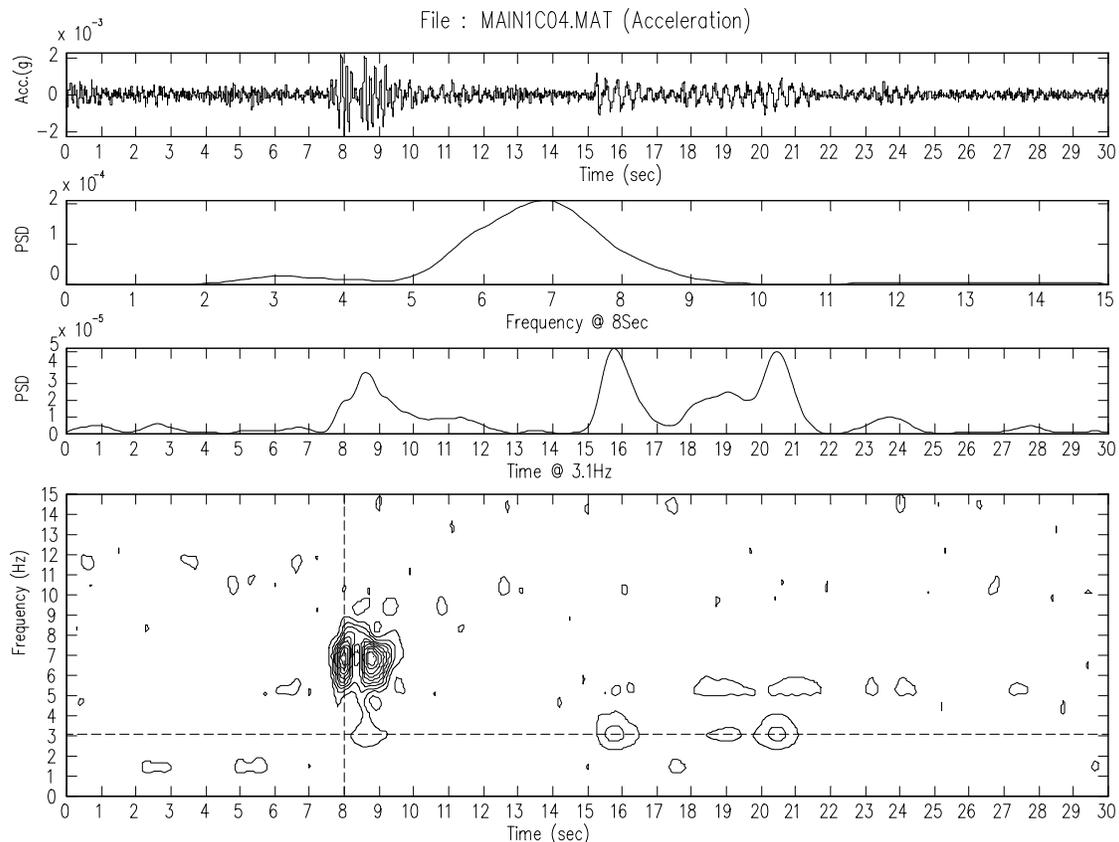
Figure 6. 2D Spectrogram of recorded dam acceleration
