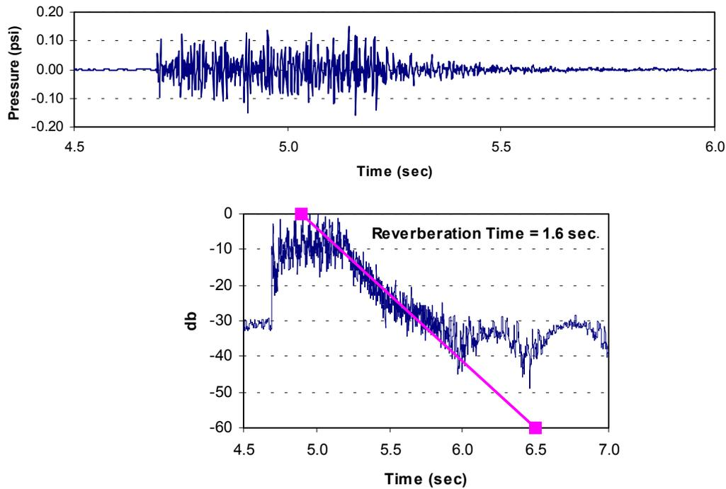
**Figure 8. Measured reverberation time at Longyangxia Dam**
